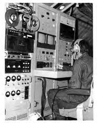
AT THE ALOTS console inside the aircraft is Al Watts (1255). Operator locates a target on one of the two TV screens above him and locks the tracking cameras on it. Just before impact he starts the ciné camera which records the event.
